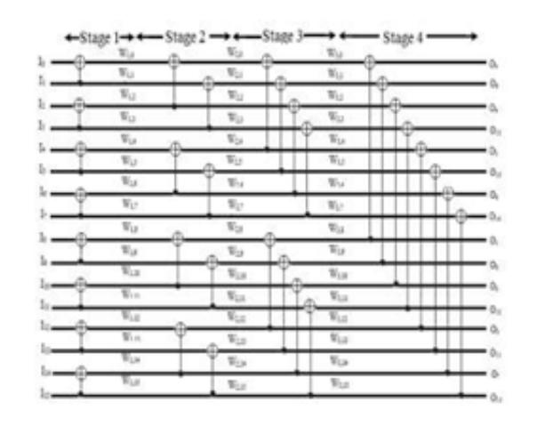
Fig.1 Fully parallel 16-bit polar encoder architecture [1]
