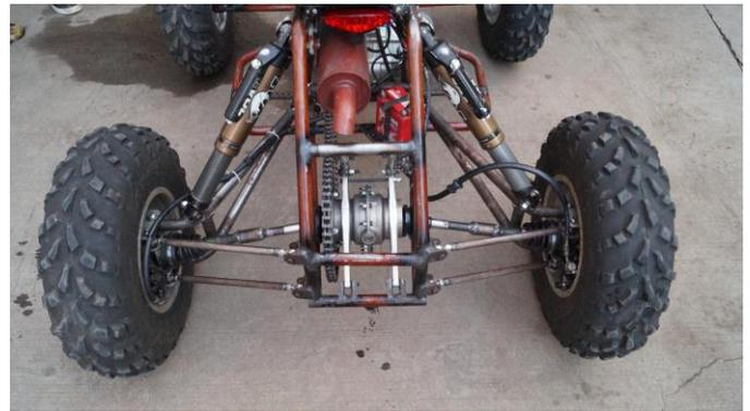
Fig 7- Three link suspension on quad bike
