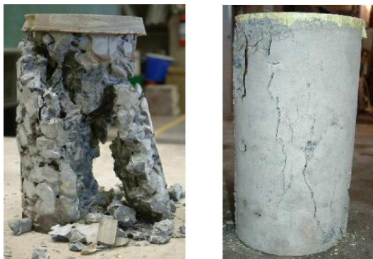
Figure 1 – Shows the shear failure mechanism of the Permeable concrete (left) and conventional concrete (right) after compressive strength testing
