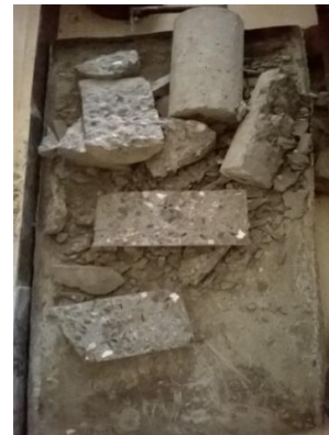
Figure 3 – The failure of the Permeable concrete after an Indirect Tensile Test
