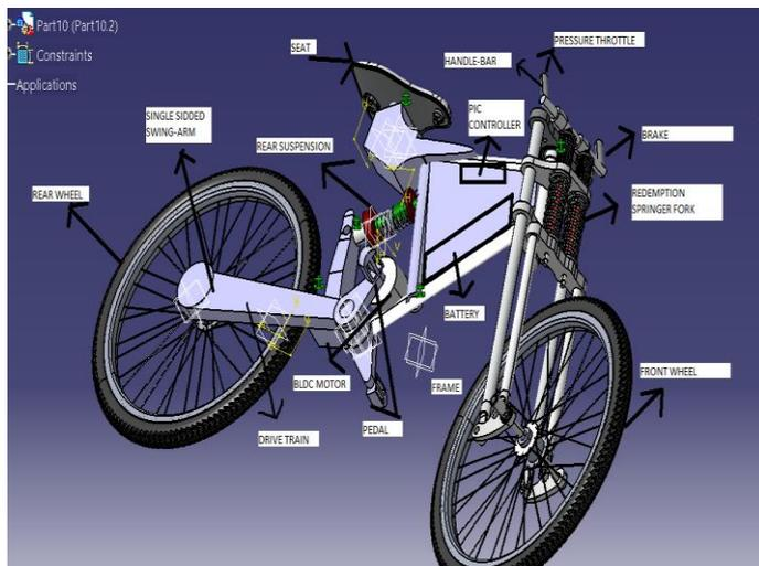
(FIG.2.2.1 SHOWS CONSTRUCTION OF "DEMON")
