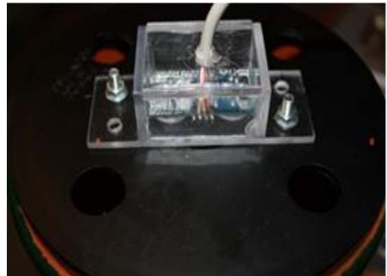
Fig 4. Instalment of ultrasonic sensor on the top of the container
