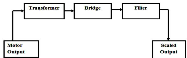
Fig -3.3: Self-Made Voltage Sensor
