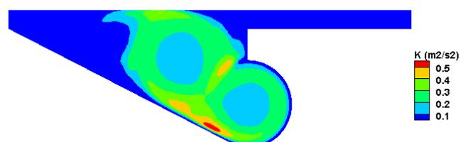
Fig -10: Turbulent kinetic energy distribution in the combustion chamber (1 ms)
