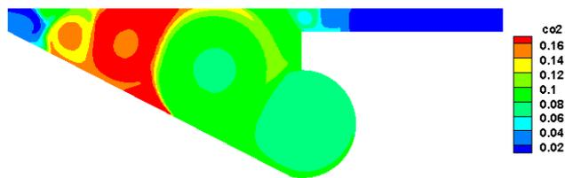
Fig -12: CO<sub>2</sub> mole fraction distribution in the combustion chamber (0.3 ms)
