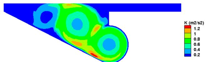
Fig -9: Turbulent kinetic energy distribution in the combustion chamber (0.5 ms)
