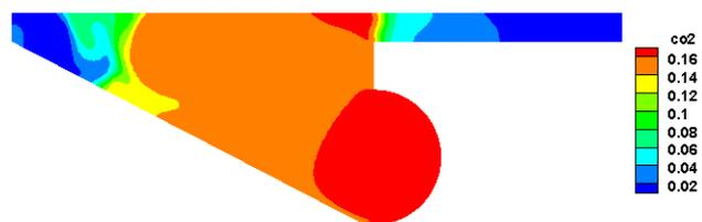
Fig -14: CO<sub>2</sub> mole fraction distribution in the combustion chamber (1 ms)
