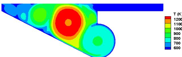
Fig -5: Temperature distribution in the combustion chamber (0.5 ms)
