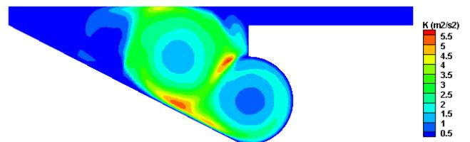
Fig -8: Turbulent kinetic energy distribution in the combustion chamber (0.3 ms)
