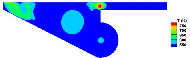
Fig -6: Temperature distribution in the combustion chamber (1 ms)
