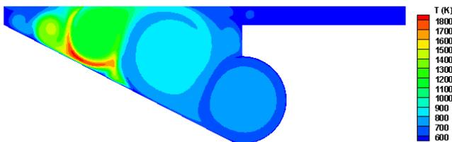
Fig -3: Temperature distribution in the combustion chamber (0.1 ms)
