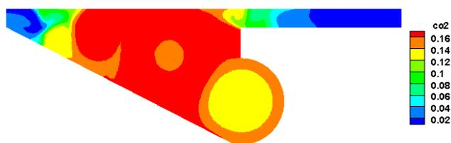
Fig -13: CO<sub>2</sub> mole fraction distribution in the combustion chamber (0.5 ms)
