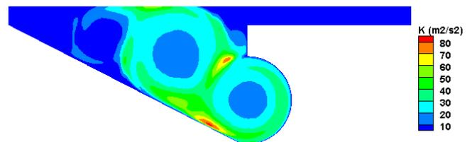
Fig -7: Turbulent kinetic energy distribution in the combustion chamber (0.1 ms)
