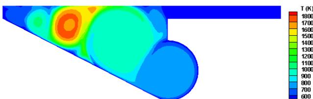
Fig -4: Temperature distribution in the combustion chamber (0.3 ms)
