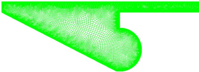
Fig -2: mesh diagram of the combustion chamber for highest resolution
