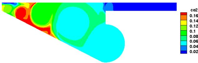
Fig -11: CO<sub>2</sub> mole fraction distribution in the combustion chamber (0.1 ms)
