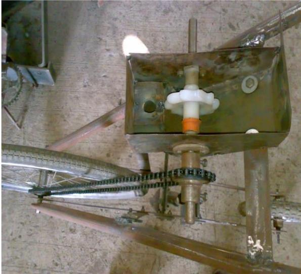
Fig.2.1 Seed Metering Mechanism
