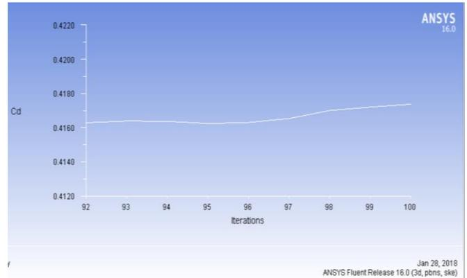
Graph 1. Iterations of drag coefficient for profile EPPLER863
