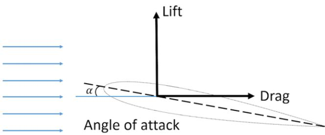
Figure 2. lift and drag components of airfoil
