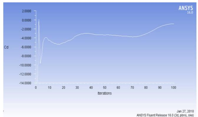
Graph 2. Iterations of drag coefficient for profile EPPLER863 with one fourth trailing edge removed
