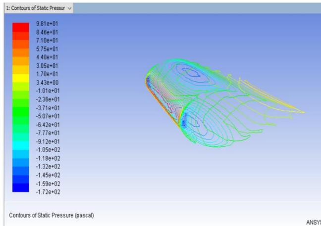
**Contour 1.** Static pressure variation for profile EPPLER863
