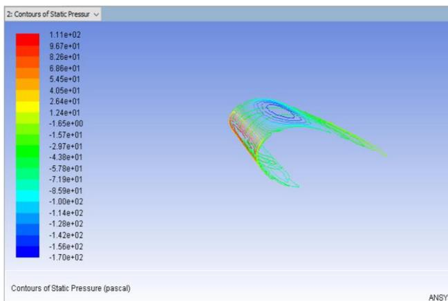
**Contour 2.** Static pressure variation for profile EPPLER863 with one fourth trailing edge removed
