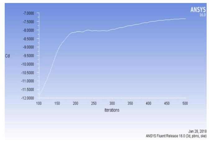
Graph 3. Iterations of drag coefficient for profile Lenz2
