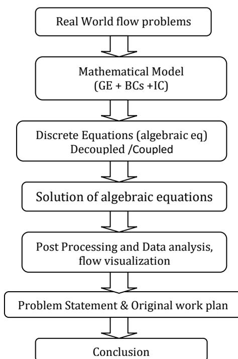
Fig.1.1. Steps of CFD Analysis diagram
