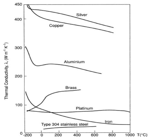
Fig.1.4. variation of thermal conductivity of metals with temperature
