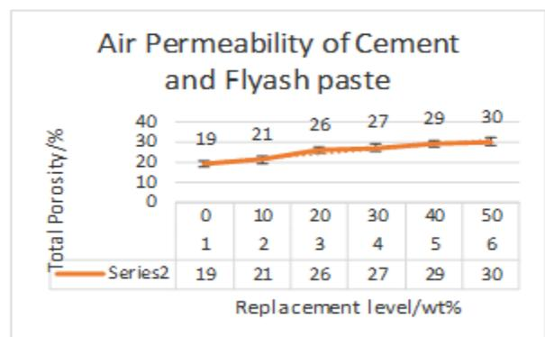
Fig 3. Air-Permeability of the cement and flyash paste
