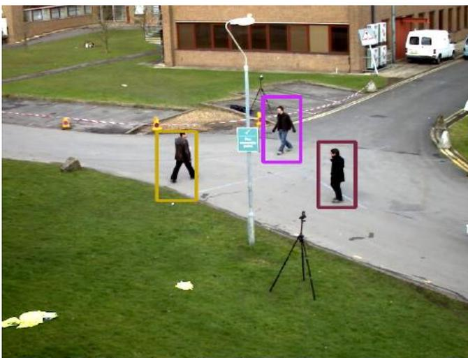
**Fig -3:** Human detection and tracking from a video
