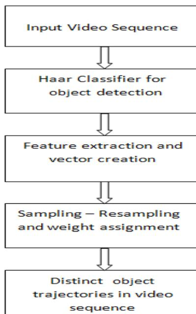
Fig -1: Phases of object detection and tracking from a video input
