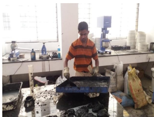
Figure 5.3 Hand mixing of CLSM
