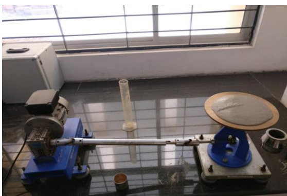
Figure 5.1 Conducting Flow table test
