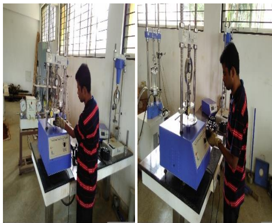
Figure 5.6, 5.7 Conducting Unconfined Compression Test
