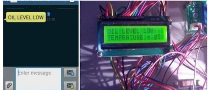
Fig-8: Oil level low detection
