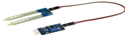
Soil Humidity Sensor Hygrometer
