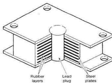
Fig -1: Lead Rubber Bearings
