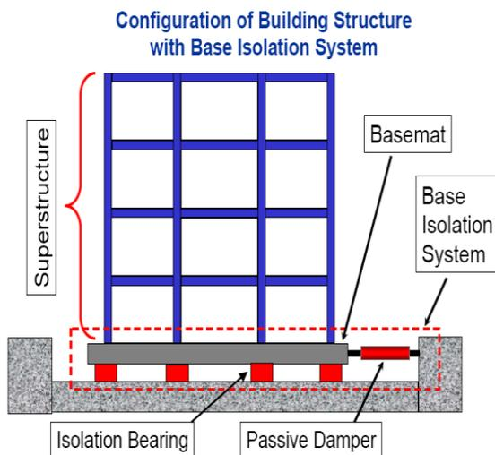
Fig-1: Building structure with Base Isolation system
