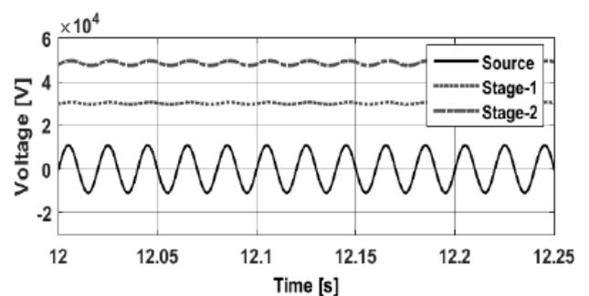
Fig. 5 Voltages of Source and Stage-1, 2
