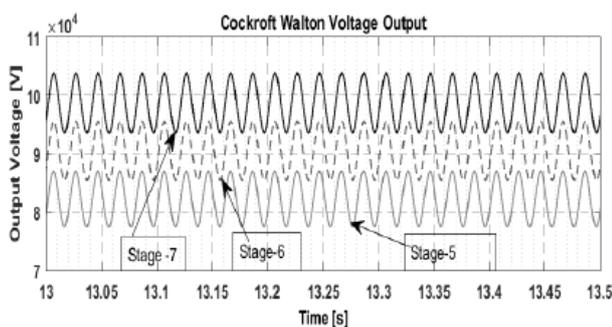
Fig. 7 Ripple Voltage Level of Output Stages
