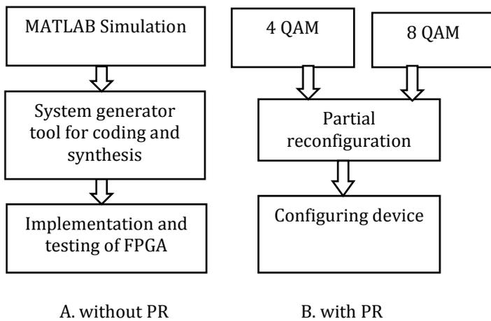
Fig. 4. Design Flow for System Implementation
