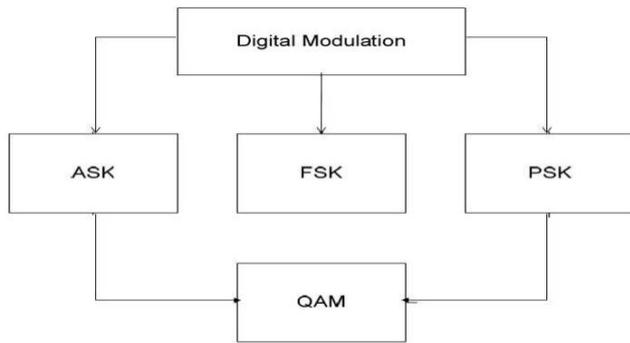
Fig. 1: Construction of QAM
