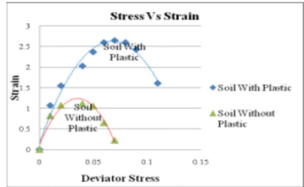
**Figure-3** Deviator stresses vs. strain for tri-axial test
