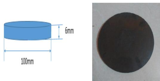
Fig- 2: Test specimen for thermal conductivity
