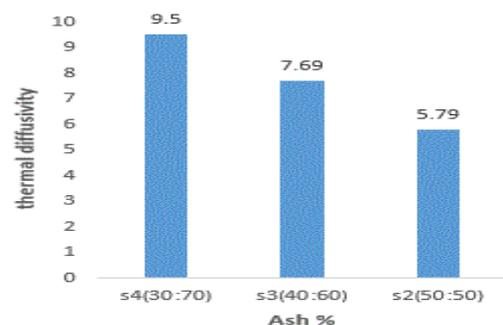
Fig-10: shows the variation of thermal diffusivity for different composition of 1- 150µm size ash
