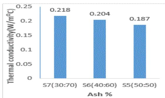
Fig-7: shows the variation of thermal conductivity For different composition of 150-325µm size ash
