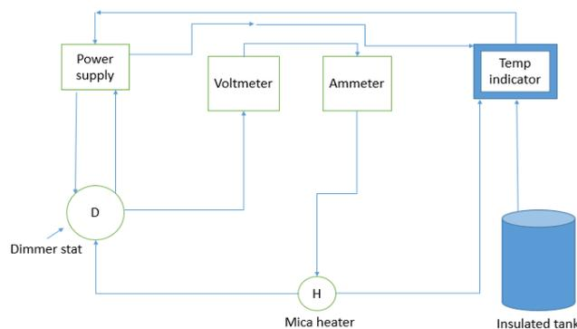
**Fig- 5:** Electric flow diagram of the specific heat test setup
