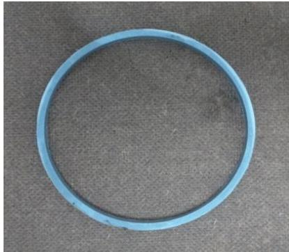
Fig- 1: Mould used for specimen preparation
