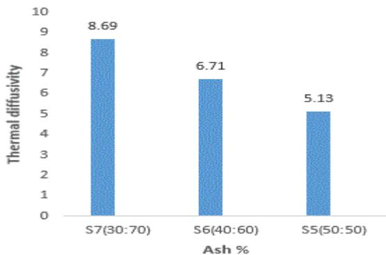
Fig-11: shows the variation of thermal diffusivity for different composition of 150-325µm size ash
