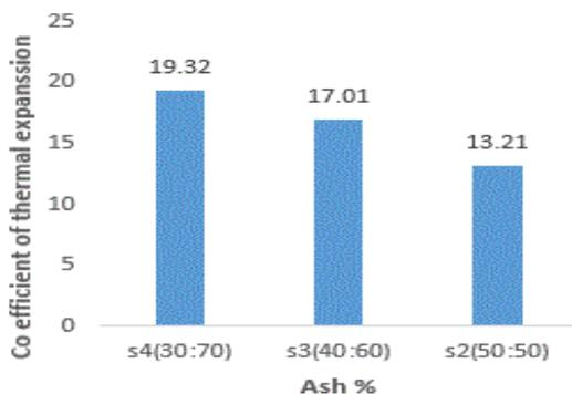
Fig-12: shows the variation of Co-efficient of thermal expansion of the composite material with different weight fractions of bagasse ash.
