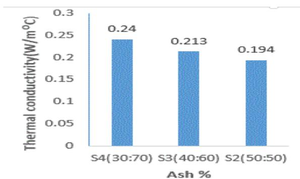
Fig-6: shows the variation of thermal conductivity For different composition of 1-150µm size ash
