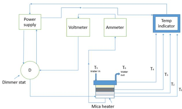
**Fig-4:** Electrical flow diagram of the thermal conductivity test setup
