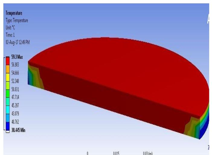
Fig-14: shows the contour plot temperature distribution along the composite(1-150µm size,50BFA:50 Epoxy) with considering convection effect
