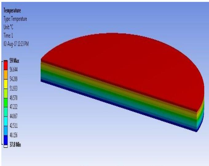
**Fig-15:** shows the contour plot temperature distribution along the composite (150-325 $\mu$ m size, 50BFA:50 Epoxy) without considering convection effect
