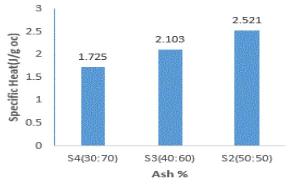
Fig-8: shows the variation of specific heat capacity for different composition of 1- 150µm size ash
