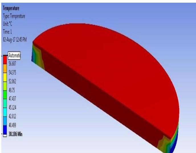
**Fig-16:** shows the contour plot temperature distribution along the composite (150-325 $\mu$ m size, 50BFA:50 Epoxy) with considering convection effect
