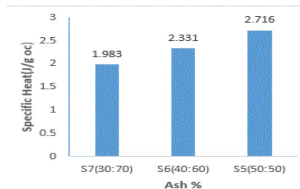
Fig-9: shows the variation of specific heat capacity for different composition of 150-325µm size ash
