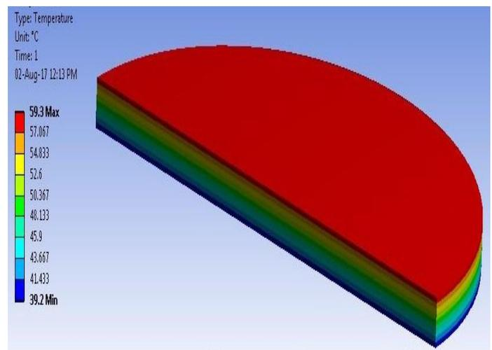
Fig-13; shows the contour plot temperature distribution along the composite (1-150µm size, 50BFA: 50 Epoxy) without considering convection effect
