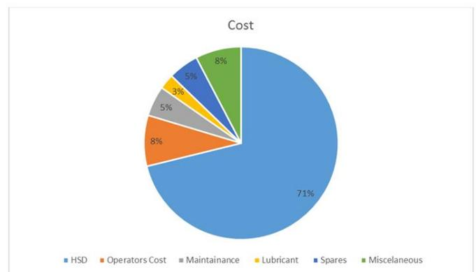
**Chart -4:** Cost Break-up of O & M of Bitumen Sprayer for Production
