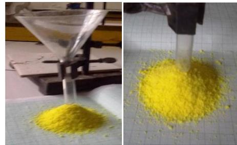
Fig 1: measuring angle of repose
