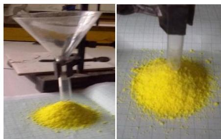
Fig 1: measuring angle of repose
