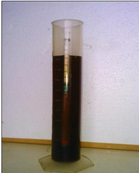
Fig2: Hydrometer for measurement of Specific Gravity
