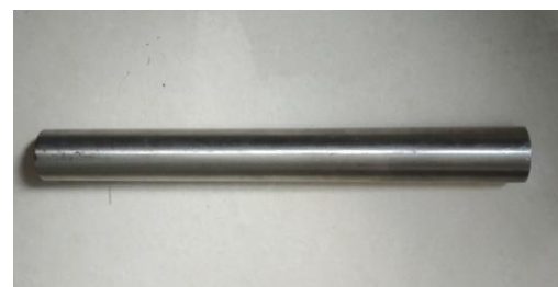
Fig -2: Photographic view of Inconel 718 bar
