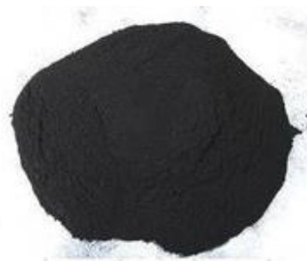
**Fig -2:** Molybdenum disulphide (MoS<sub>2</sub>) in form of nano powder
