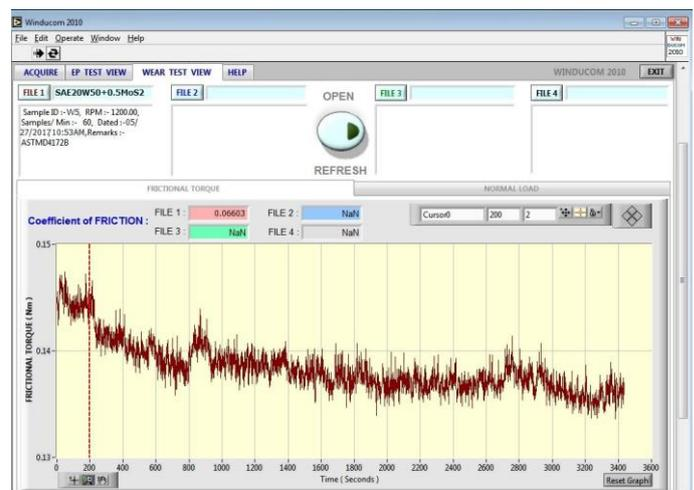
**Graph -1:** of frictional torque (Nm) Vs time (sec) for sample W5 (Base oil +0.5%MoS<sub>2</sub>)
