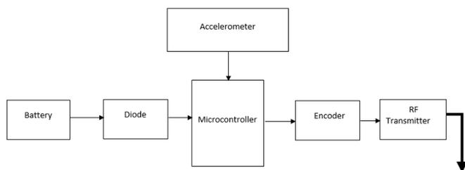
An RF transmitter module can transmit a radio wave and modulate that wave to carry data. Transmitter modules are usually implemented alongside a micro controller which will provide data to the RF module which is transmitted. RF transmitters are usually subject to regulatory requirements which dictate the maximum allowable transmitter power output.
