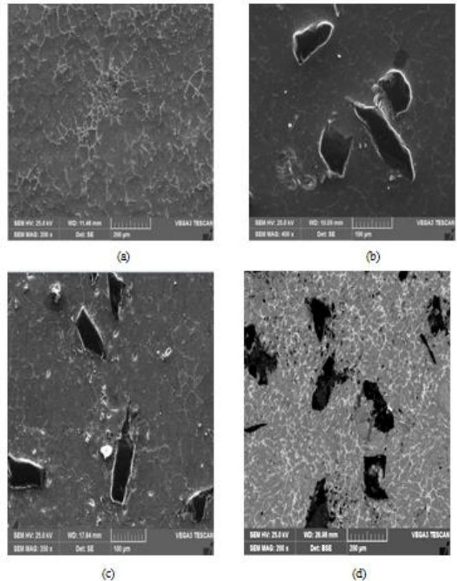
Figure 1: Shows the SEM photographs of (a) as cast AA7030 alloy (b) AA7030-3% B<sub>4</sub>C (c) AA7030-6% B<sub>4</sub>C (d) AA7030-9% B<sub>4</sub>C composites
