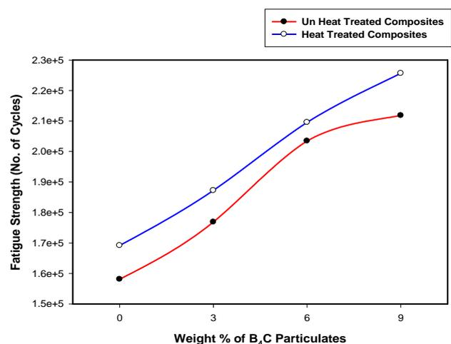
Figure 6: Fatigue strength of AA7030-B<sub>4</sub>C composites with and without heat treatment
