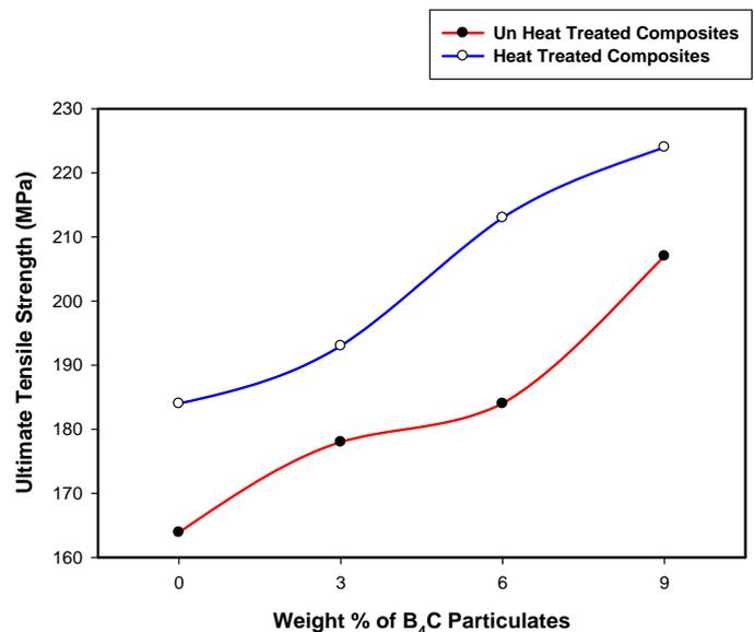
Figure 3: Ultimate tensile strength of AA7030-B<sub>4</sub>C composites with and without heat treatment
