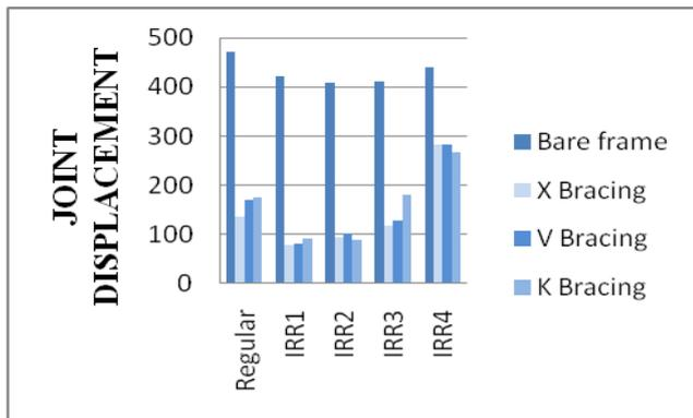
Fig.15. Comparison of joint displacement
