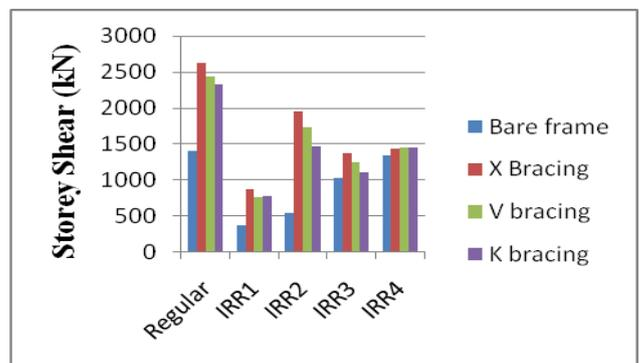
Fig.8. Comparison of storey shear in x direction
