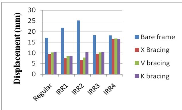
Fig.10. Comparison of displacement in x direction
