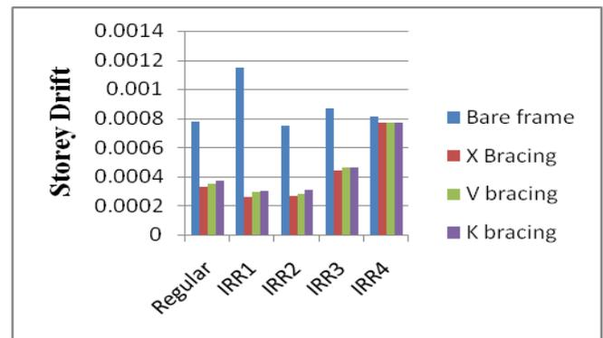
Fig.13. Comparison of storey drift in y direction
