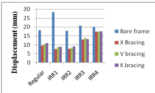
Fig.11. Comparison of displacement in y direction
