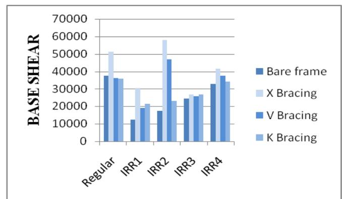
Fig.14. Comparison of base shear
