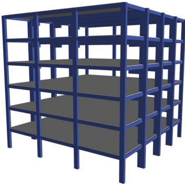
Fig.3.2 Six Storeyed RC Frame System
