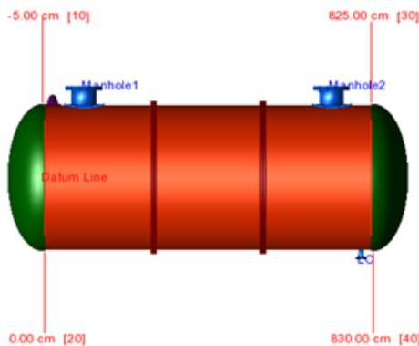
Fig-1 Mounded pressure vessel with stiffening rings
