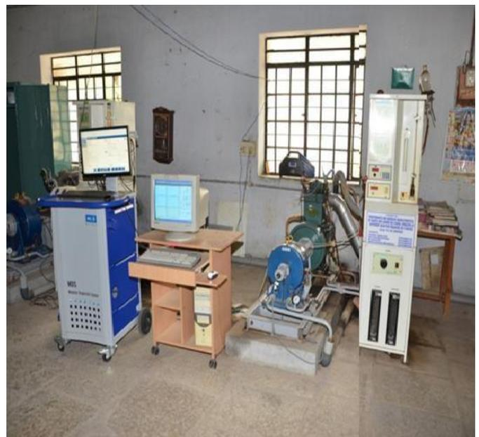
**Fig:-2.1 Engine connected with dash board**
