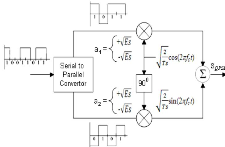
Fig. 1. Conventional block diagram of QPSK modulator.
