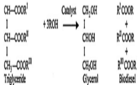
Some of the biodiesel fuels properties [6-22] are compared in Table 1. The characteristics of biodiesel are close to petroleum diesel, and, therefore, biodiesel becomes a strong candidate to replace the petroleum diesel. The molecular weight and the viscosity of vegetable oils is reduced by the conversion of vegetable oil into biodiesel through the transesterification process which increases the volatility marginally.
