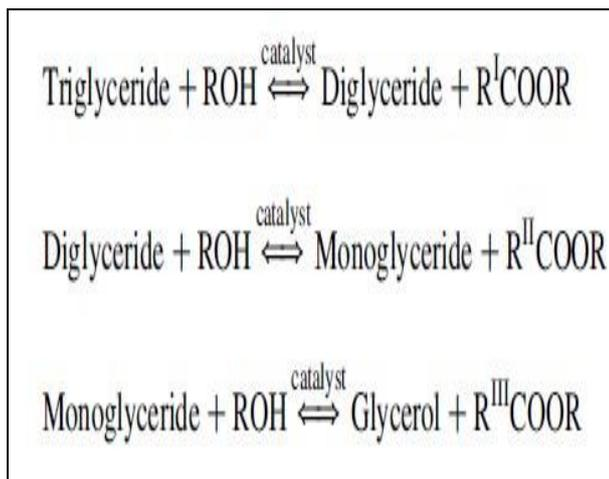
**Figure 1.** The transesterification reaction ( $\text{R}^{\text{I}}$ ,  $\text{R}^{\text{II}}$  and  $\text{R}^{\text{III}}$  long-chain hydrocarbons which may be the same or different with  $\text{R} = \text{CH}_3/\text{C}_2\text{H}_5$ )
