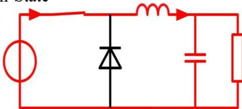
Fig -3: Buck Converter ON State
