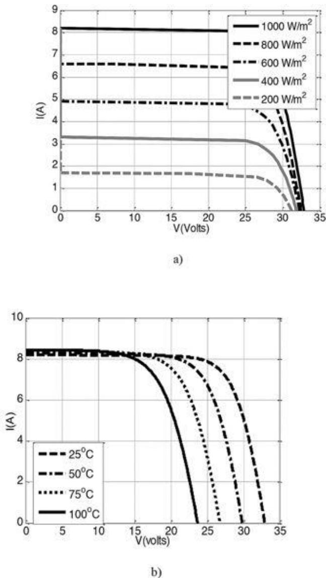
Fig -1 : (a) I-V characteristics of PV panel for different irradiance level. (b) I-V characteristics corresponding to different temperature.
