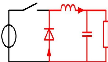
Fig -4: Buck Converter OFF State
