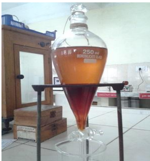
Fig 2.1: Separation of biodiesel and glycerine
