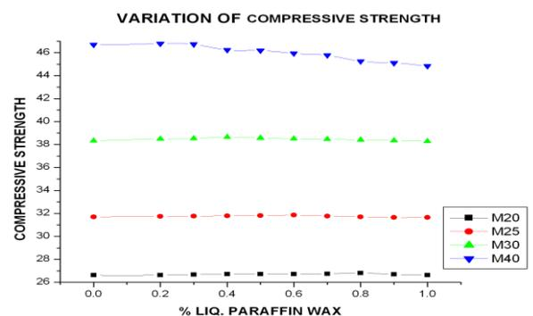
**Fig -4.1:** Variation of compressive strength for different % of LPW for grade M20, M25, M30 & M40
