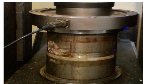
Fig 4: Load cell with strain gauges
