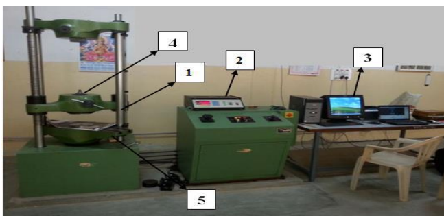
Fig-1: Electronic universal testing machine (1) Machine frame (2) Servo control unit (3) Computer control (4) Cross head (5) Lower Table
