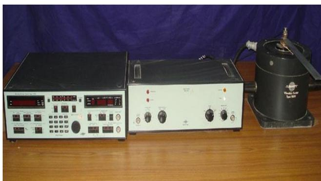
Fig 1:- Vibration Exciter With F.F.T
