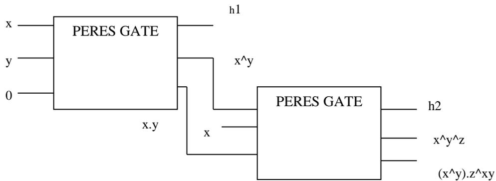
Fig. 5. Full Adder using Peres Gate
