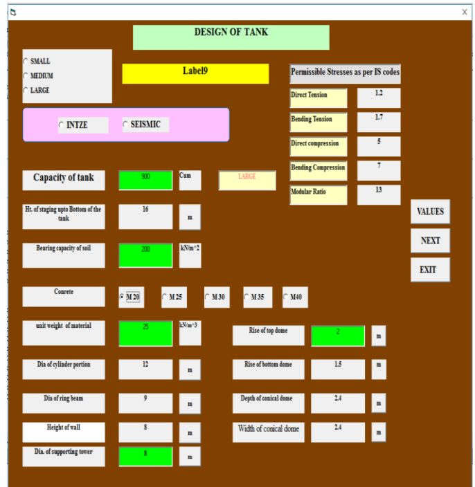
Fig-2 Screen shot showing dimensions of the Intze Water Tank in VISUAL Basic
