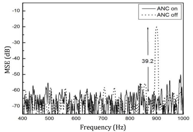
**Figure 5.** MSE of residual noise (single sinusoidal signal)
