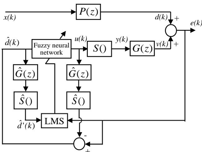
Figure 2. The proposed ANC system with saturation compensation
