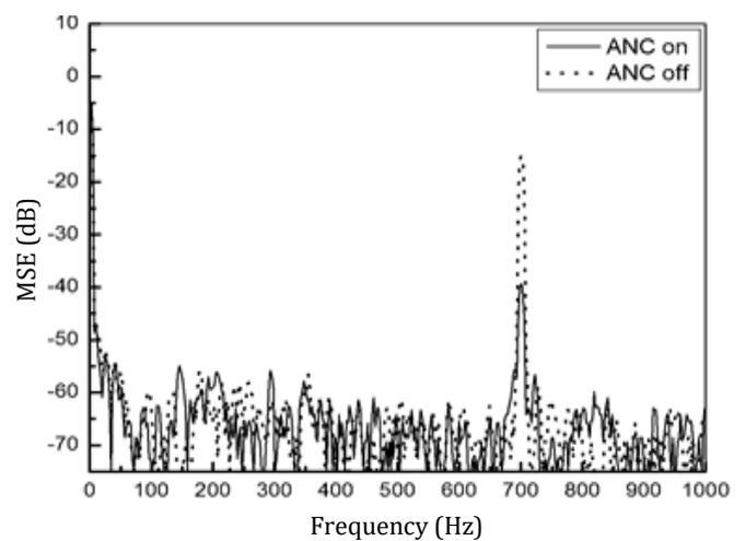
**Figure 7.** MSE of residual noise of the proposed ANC system
