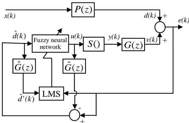
Figure 1. Diagram of adaptive feedback ANC system using fuzzy neural network
