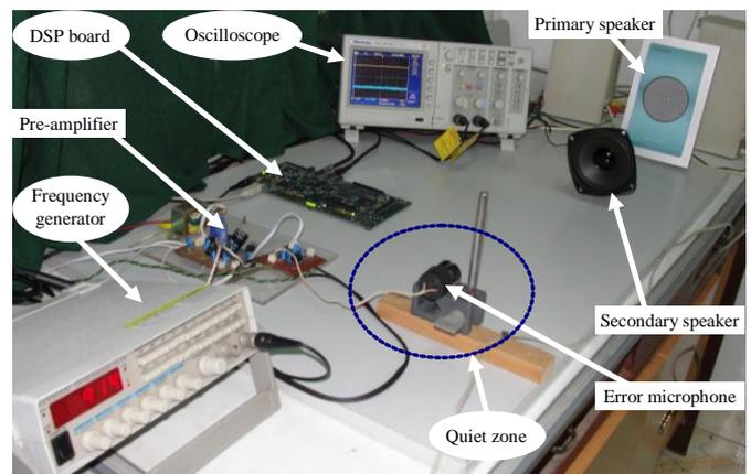
**Figure 4.** The ANC experiment setup
