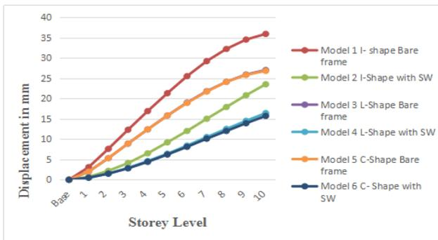
Graph No.2 Story Displacement of all models in Y-Direction in mm.
