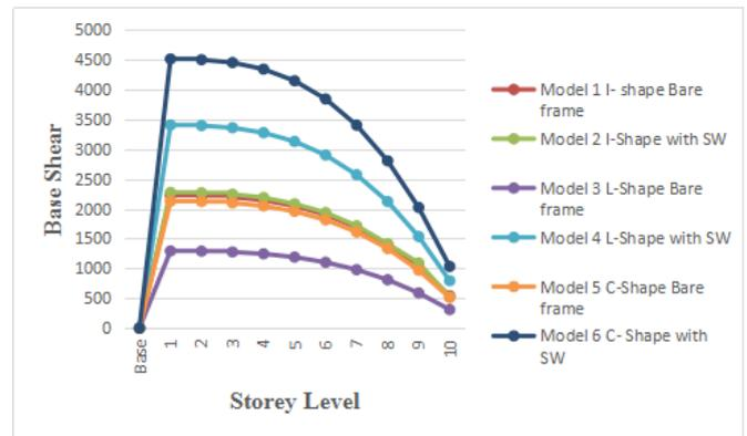
Graph No.3 Base Shear of all models in X-Direction in KN.
