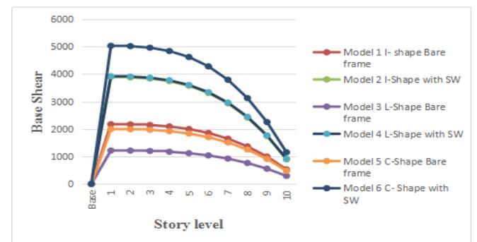
Graph No.4 Base Shear of all models in Y-Direction in KN.
