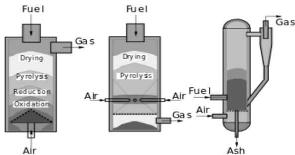
**Fig -4:** Updraft, Downdraft, Fluidized bed gasifiers
