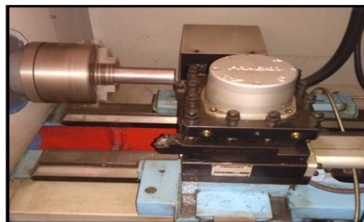
Fig.3.5: Photograph of experimental setup for turning of Inconel 825.
