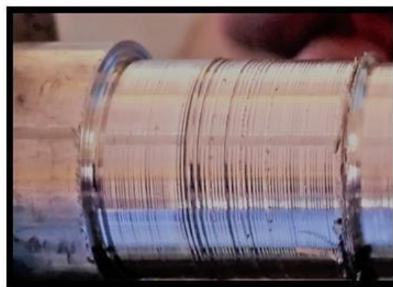
Fig.4.4(A): Variation in surface finishing of workpiece when it is machined with worn out tool
