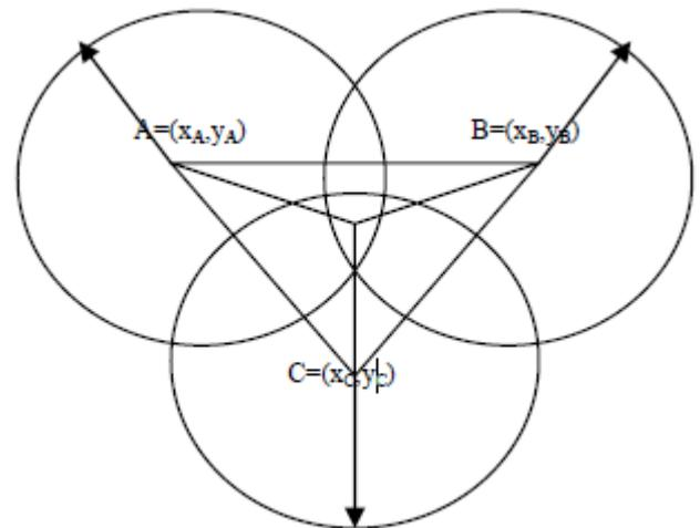
Figure-5: Position Approximation Algorithm
