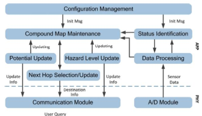
Fig 2 Architecture of the experimental testbed
