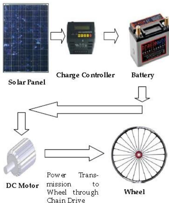
Figure 5: Diagram of solar power system
