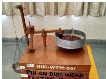
Fig. 5 Pin on Wear testing machine
