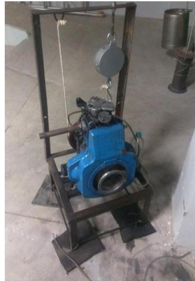
Fig.12 Engine with Rope brake Dynamometer
