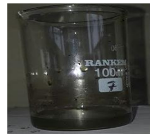
Figure 3 : Sedimentation test of Copper Oxide nanofluid.
