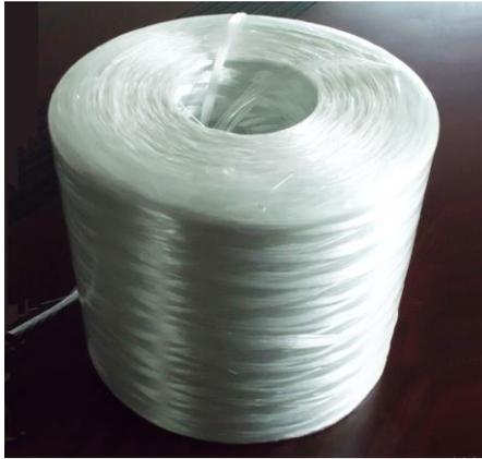
**Fig 2. Fiberglass roving**
