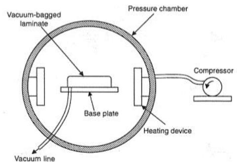
Fig 5. Bagging Setup
