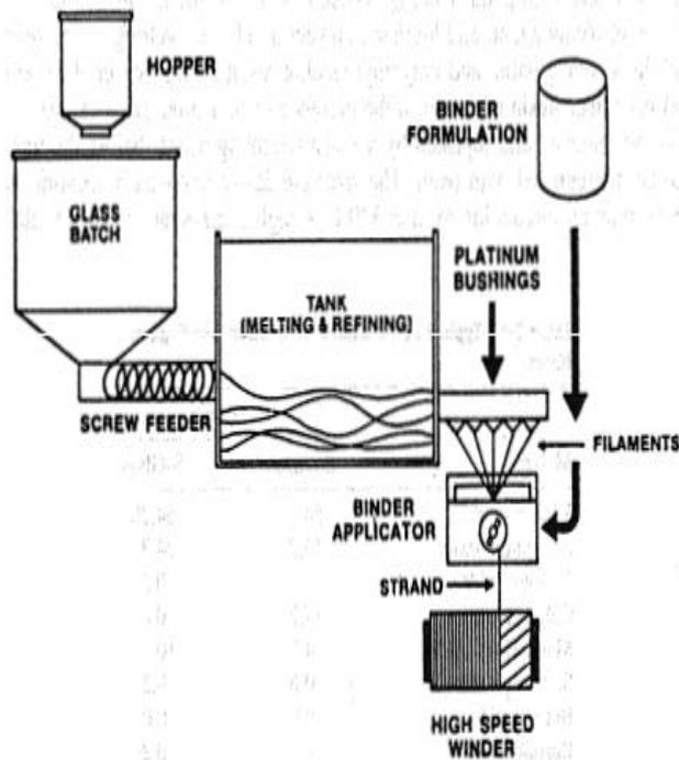
Fig1. Glass fiber production setup
